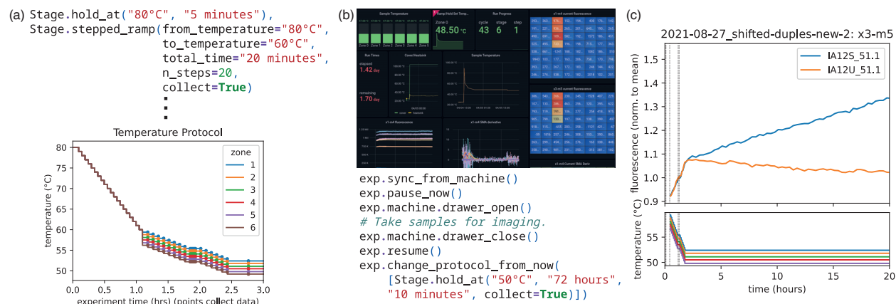
Figure 1: (a) Protocols are specified as code and can be easily plotted, as for the temperature ramp with six offset temperatures for different plate columns shown here. (b) Real-time data can be sent to open source dashboard software, such as Grafana, shown here. During runs, data can be imported and plotted, samples can be removed for imaging, and temperature schedules can be changed arbitrarily: for example, to quickly find a growth temperature in exploratory experiments. (c) Qslib offers convenient plotting of fluorescence data, and one-second-resolution temperature data, unavailable in the manufacturer's software. Here, a seeded DNA tile ribbon with a FRET pair probe grows at 51.1°C (blue), while an unseeded ribbon does not (orange); similar samples at six temperatures were run in parallel on the machine.
